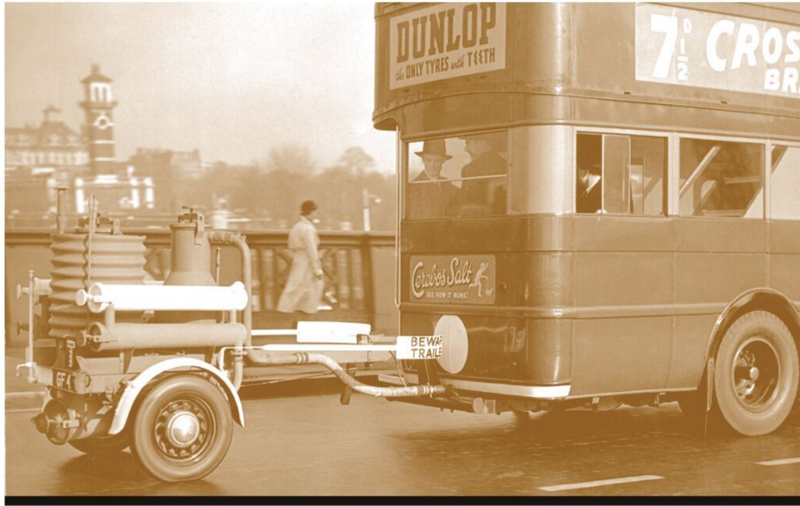
A London bus with gas generator. Here the conversion kit was put on a trailer.
