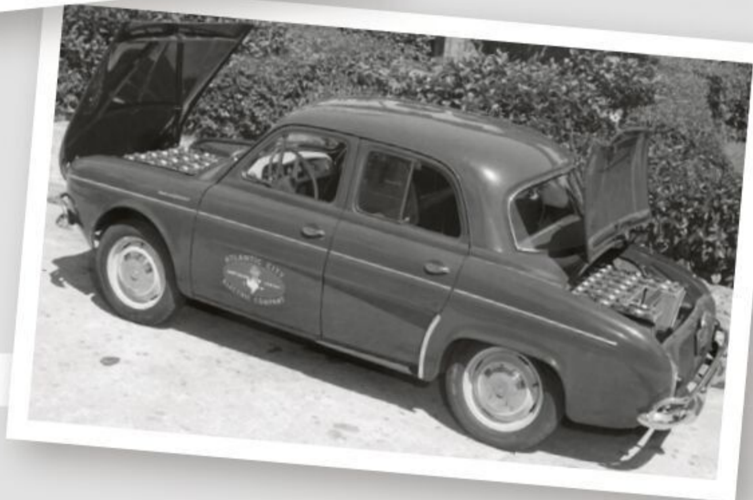
The Briggs-Stratton was a parallel hybrid, which could run solely on the gas engine, the electric motor, or a combination of both.
