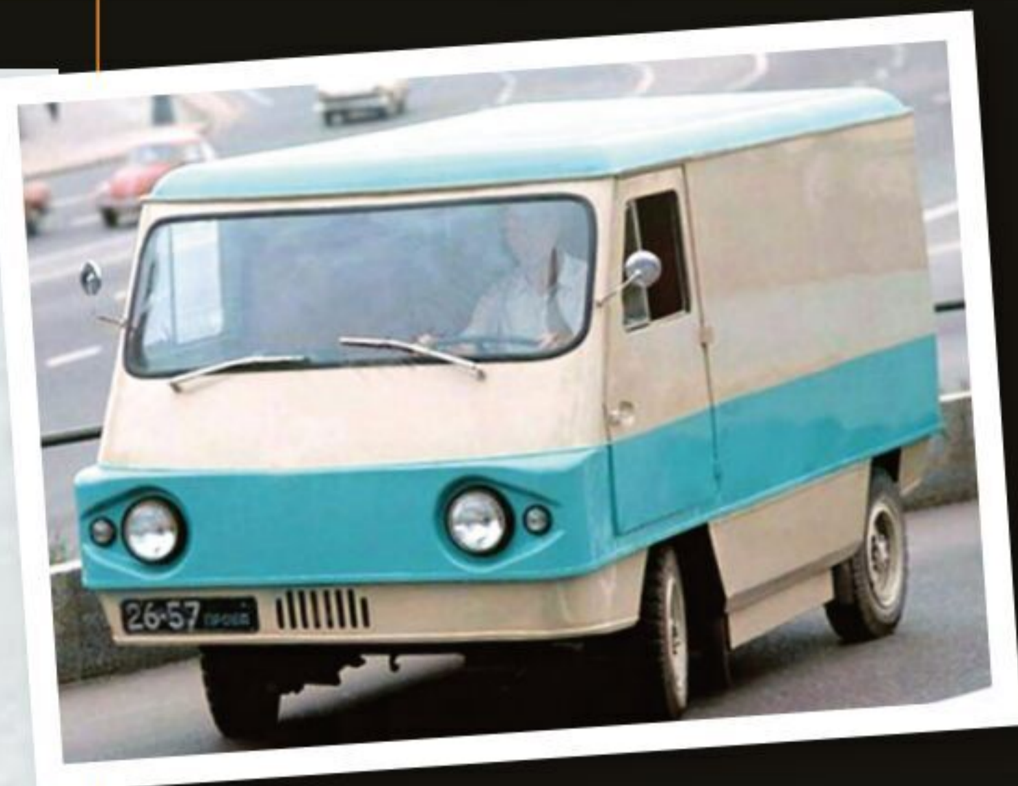
The VNIET research institute in Kaliningrad built a few prototypes between 1967 and 1970 with asynchronous AC motors.
