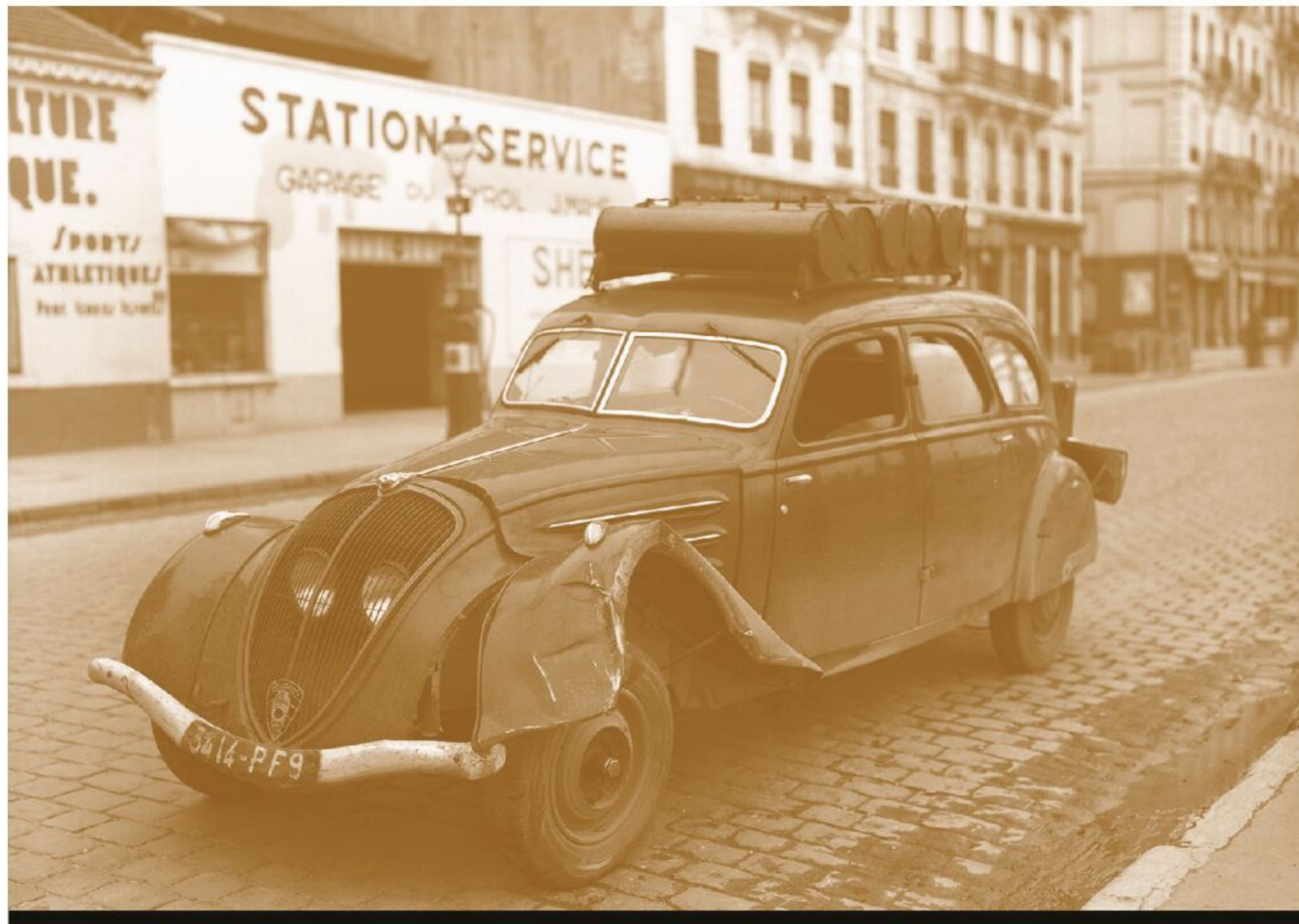
This photo was probably taken in Lyon in around 1942 showing a dented Peugeot 402 with a charcoal burner at the back and four cleaning drums on the roof.
