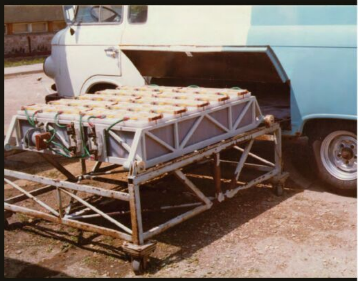
The battery pack made the Barkas very slow and unreliable.
