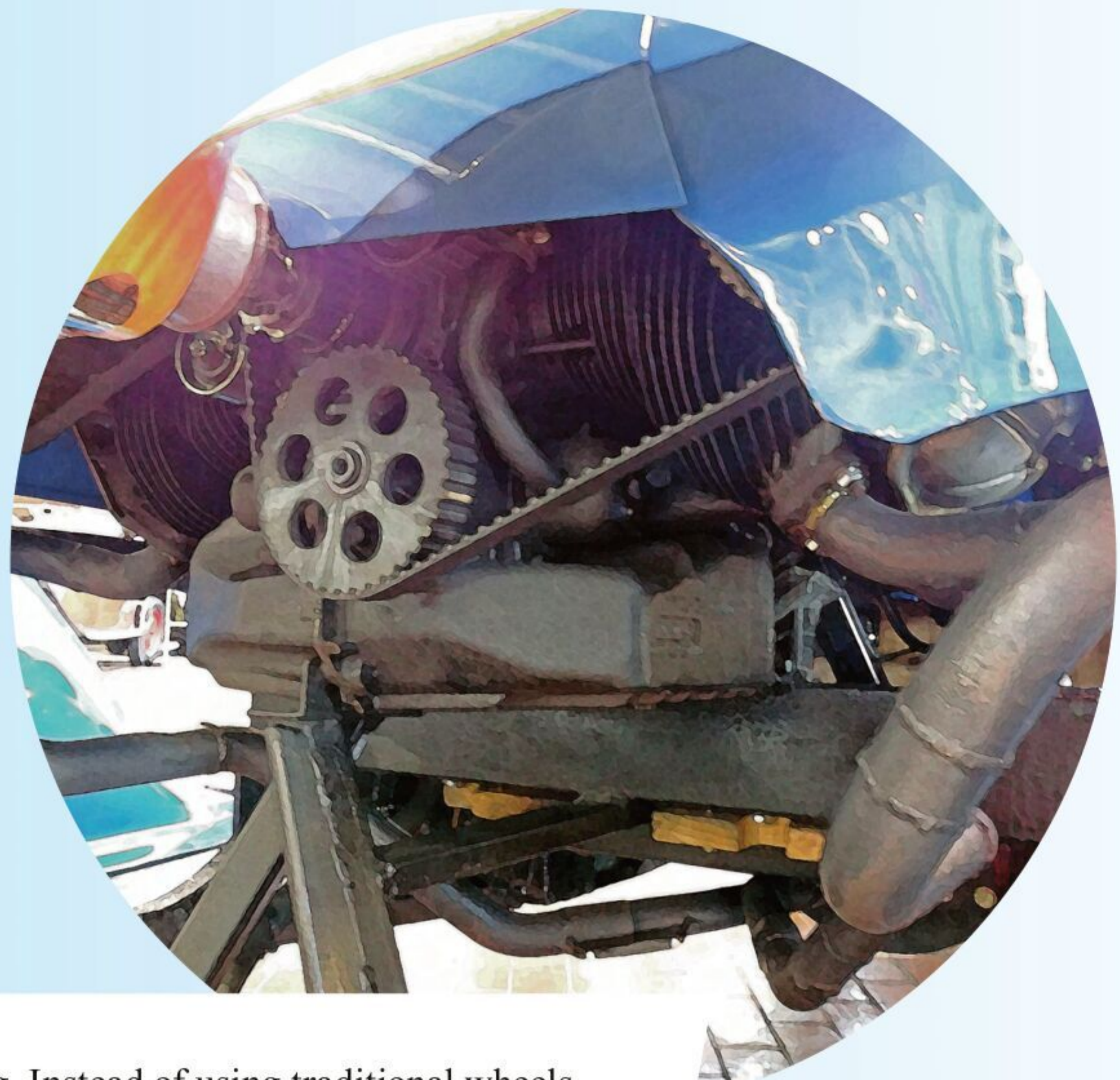
The builder of the Helicron flipped the chassis 180 degrees.
