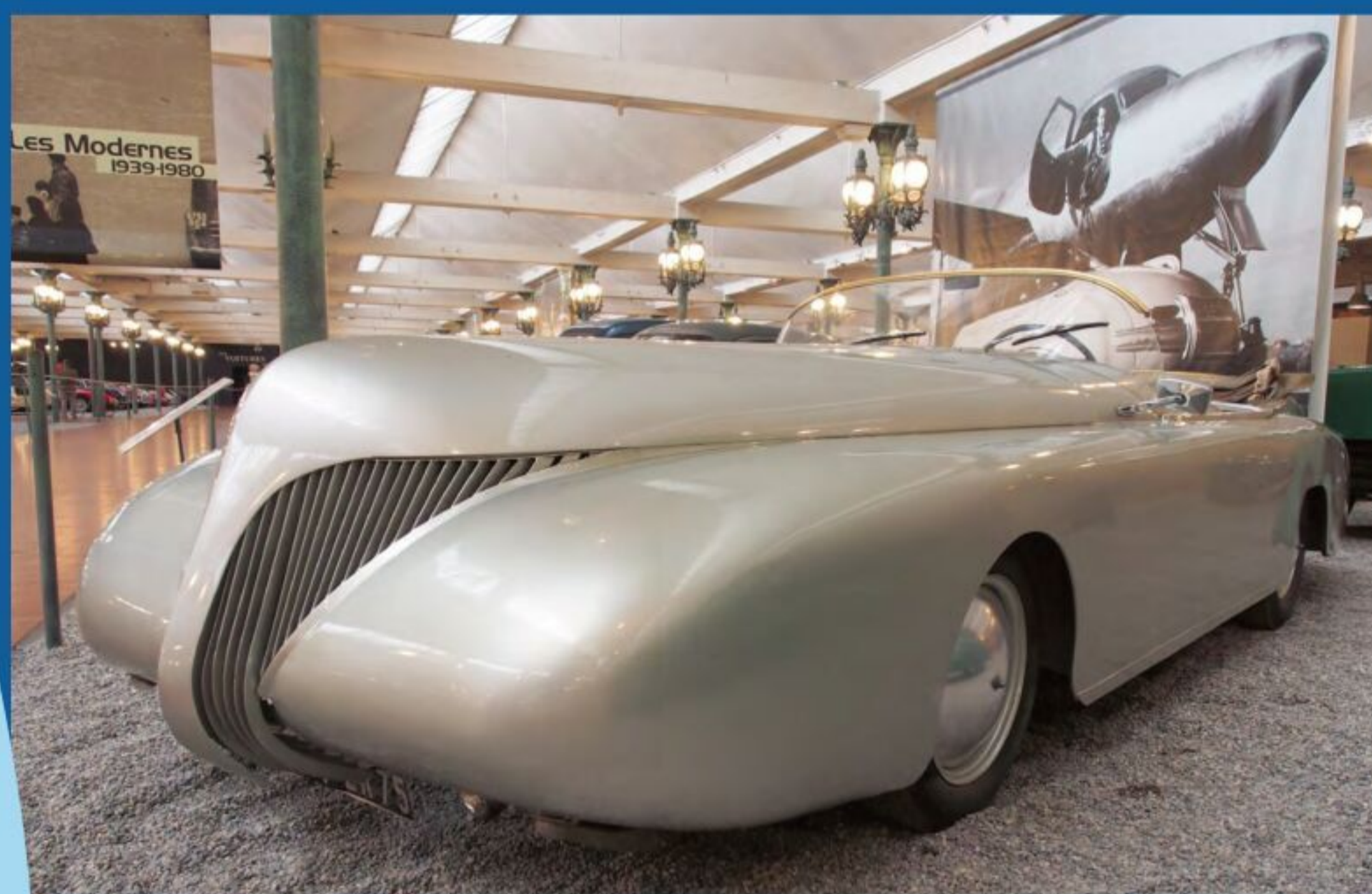
Top: The second version of La Baleine was based on a Fiat chassis and featured an electric powertrain.
