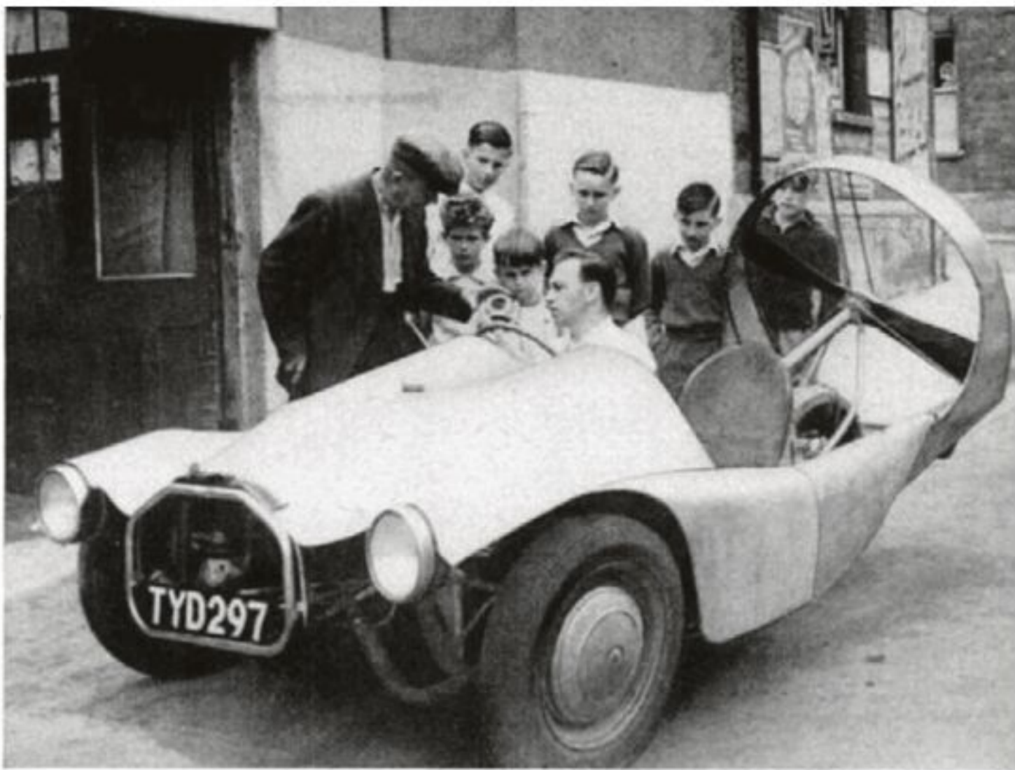
One of the few postwar propeller cars was built by Clifford Robins in the United Kingdom.
