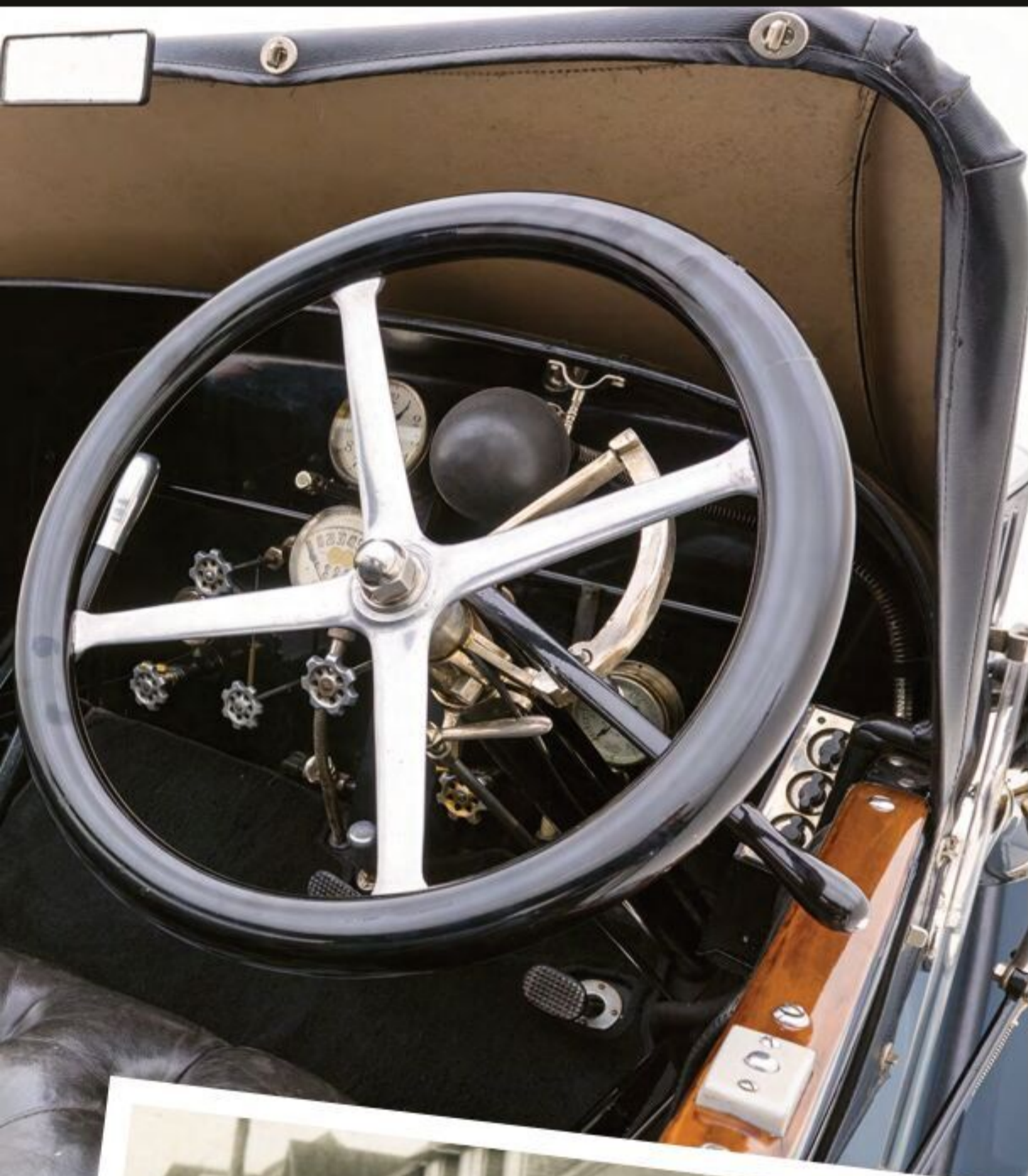
2 Instead of a standard windshield Raymond Stanley preferred a canvas covering, known as the "Cambridge Windshield".
