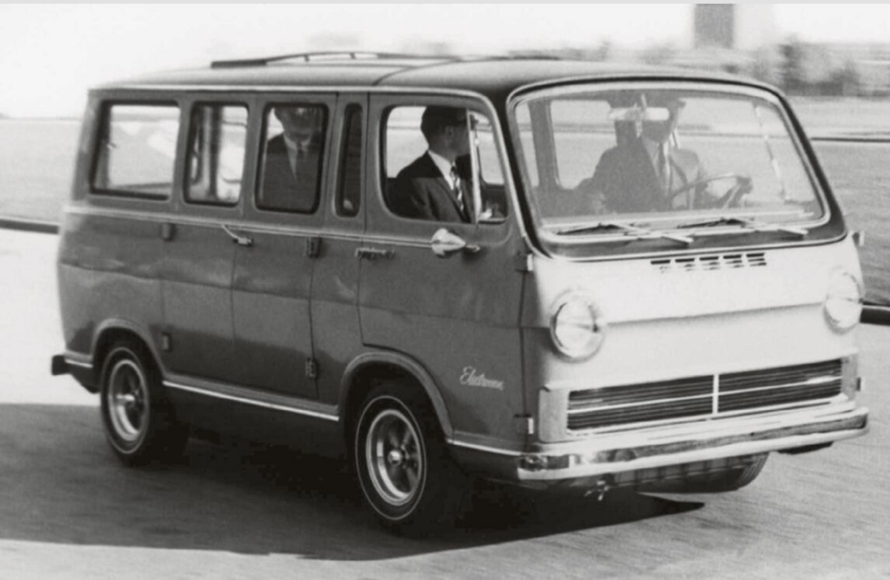
1966 GM Electrovan is credited with being the first hydrogen fuel cell car ever produced.
