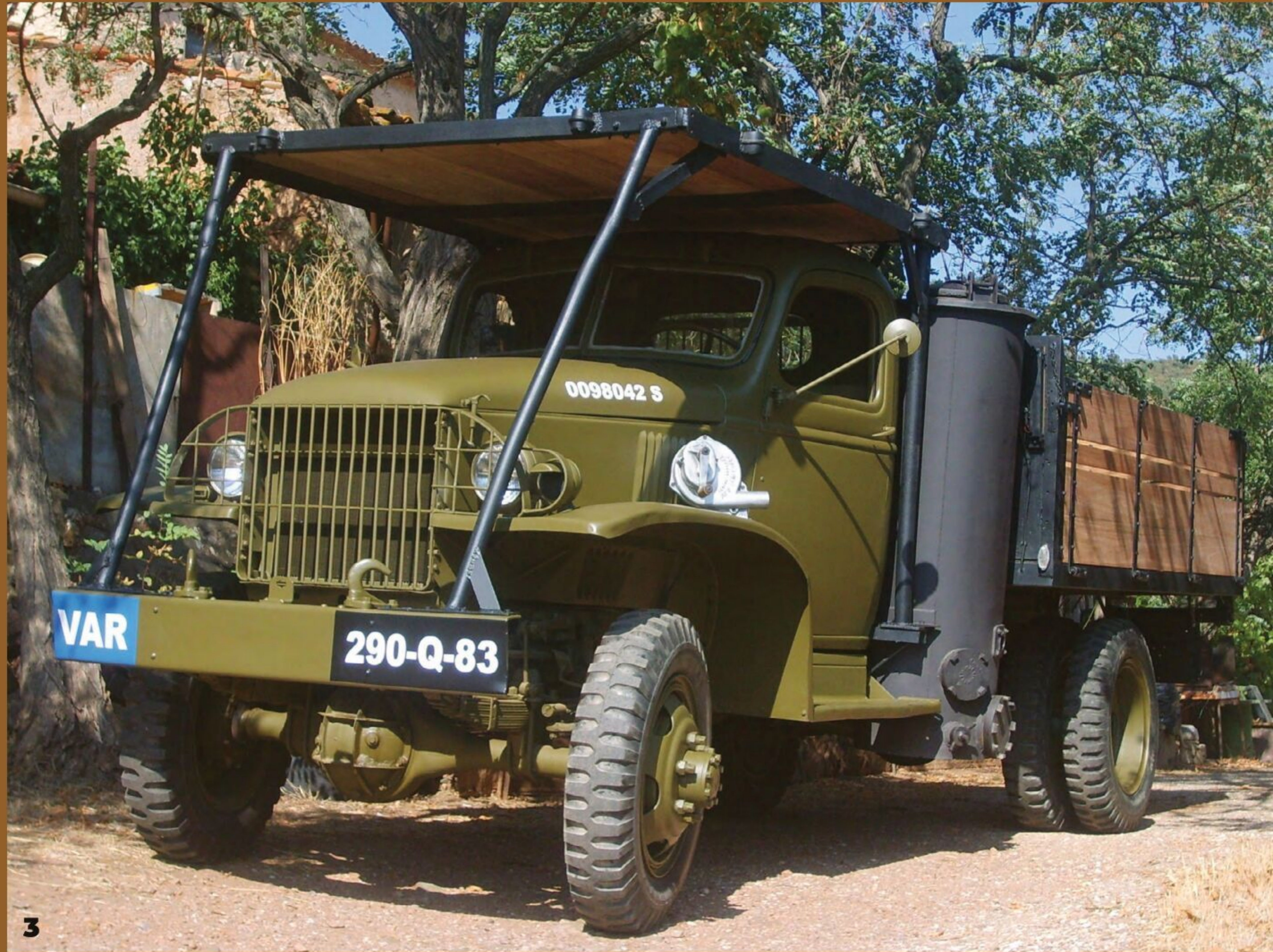
3 Bruno Grossi's restored Chevrolet truck with an Imbert generator.
