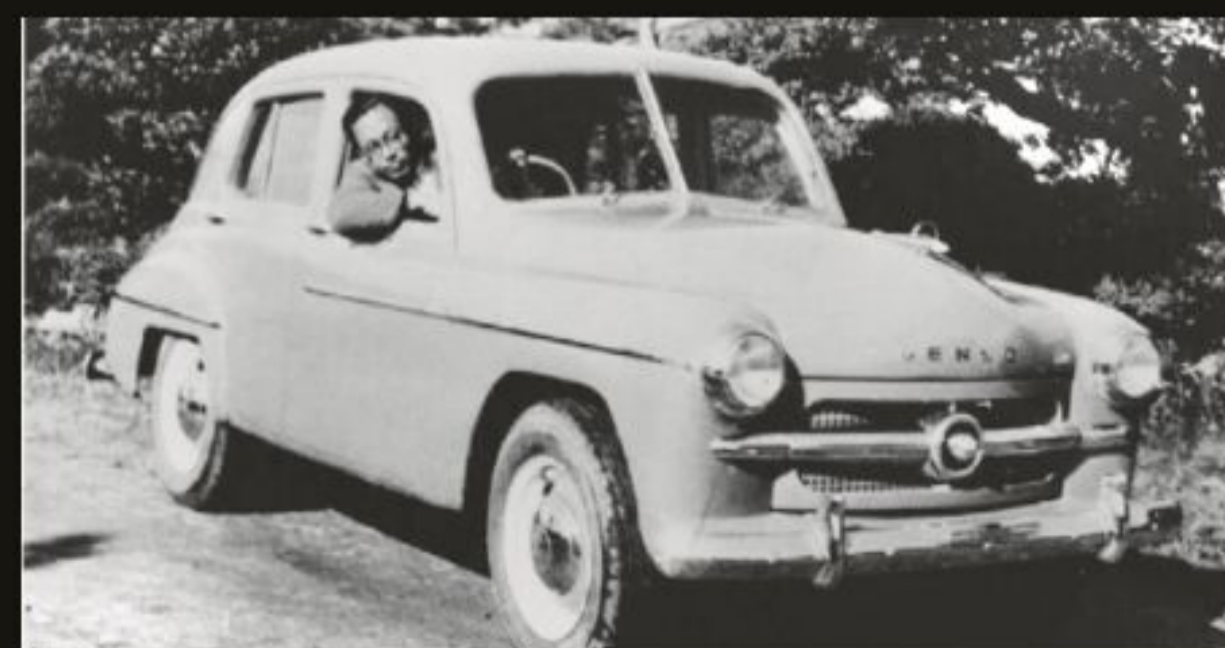
The Denso No 1 was a modified Toyopet SD, which was equipped with an electric powertrain.
