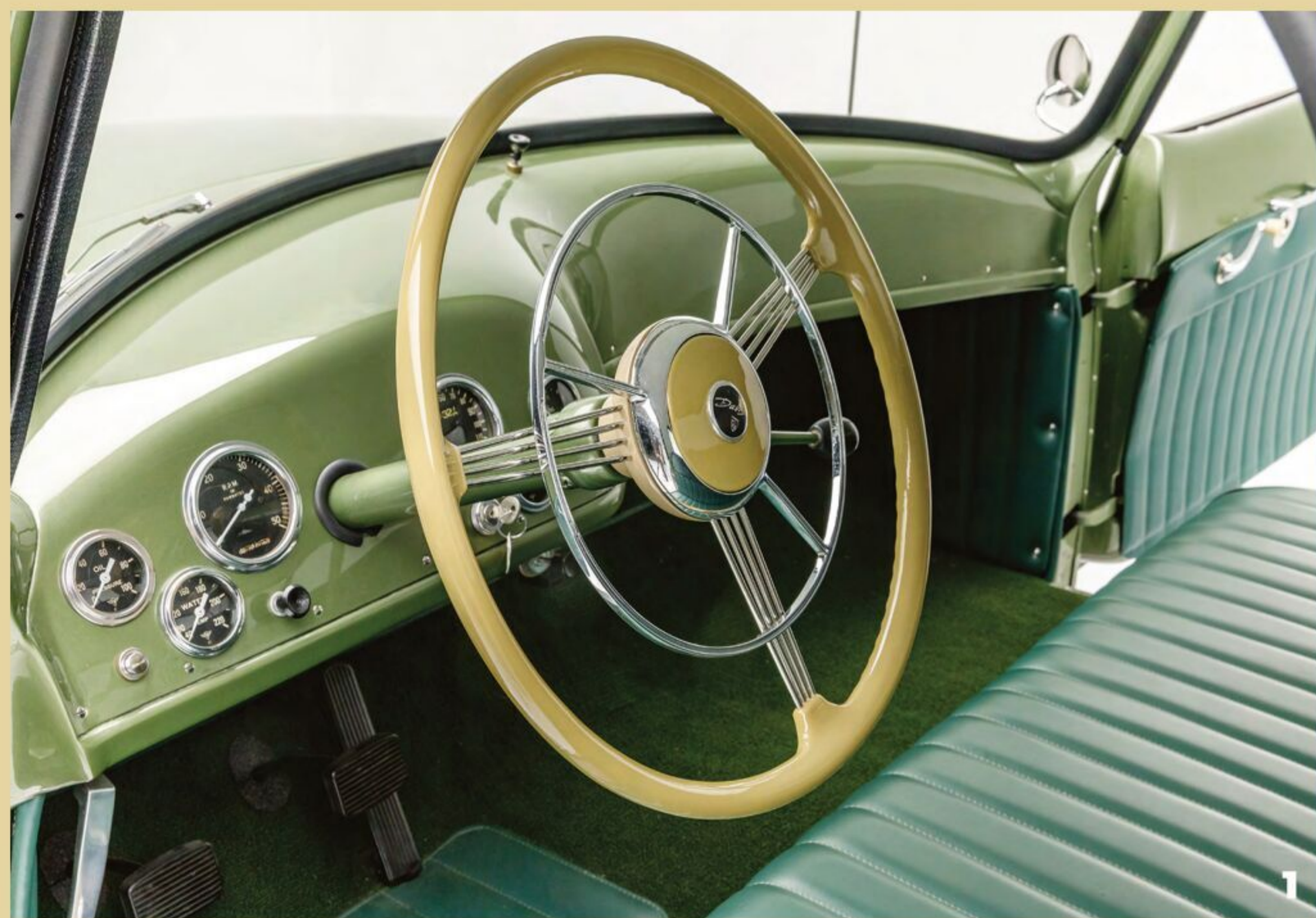
1 A switch on the dashboard operated built-in hydraulic jacks.
