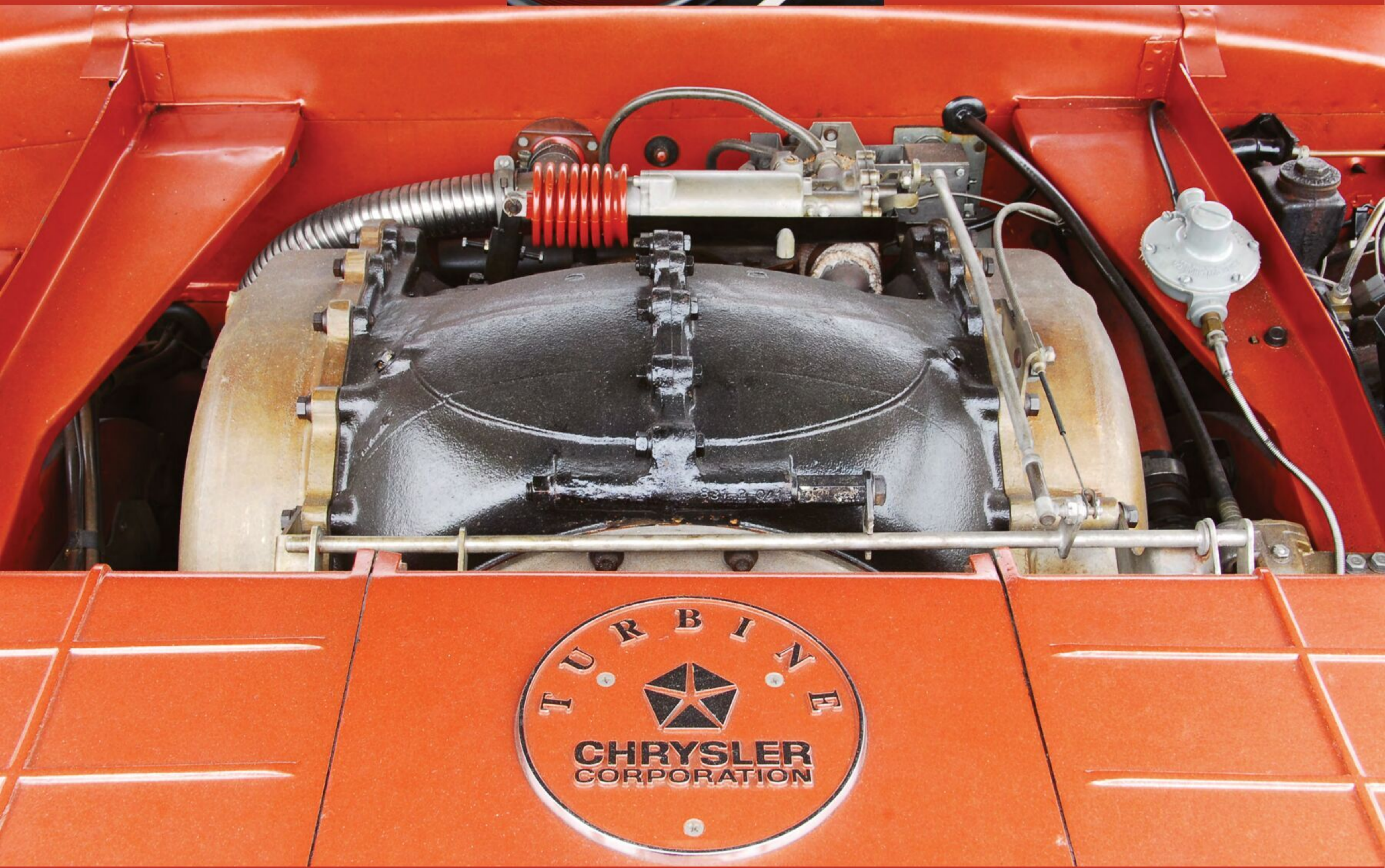
The fourth-generation Chrysler turbine engine looks something like a small nuclear reactor but produces 130 horsepower.
