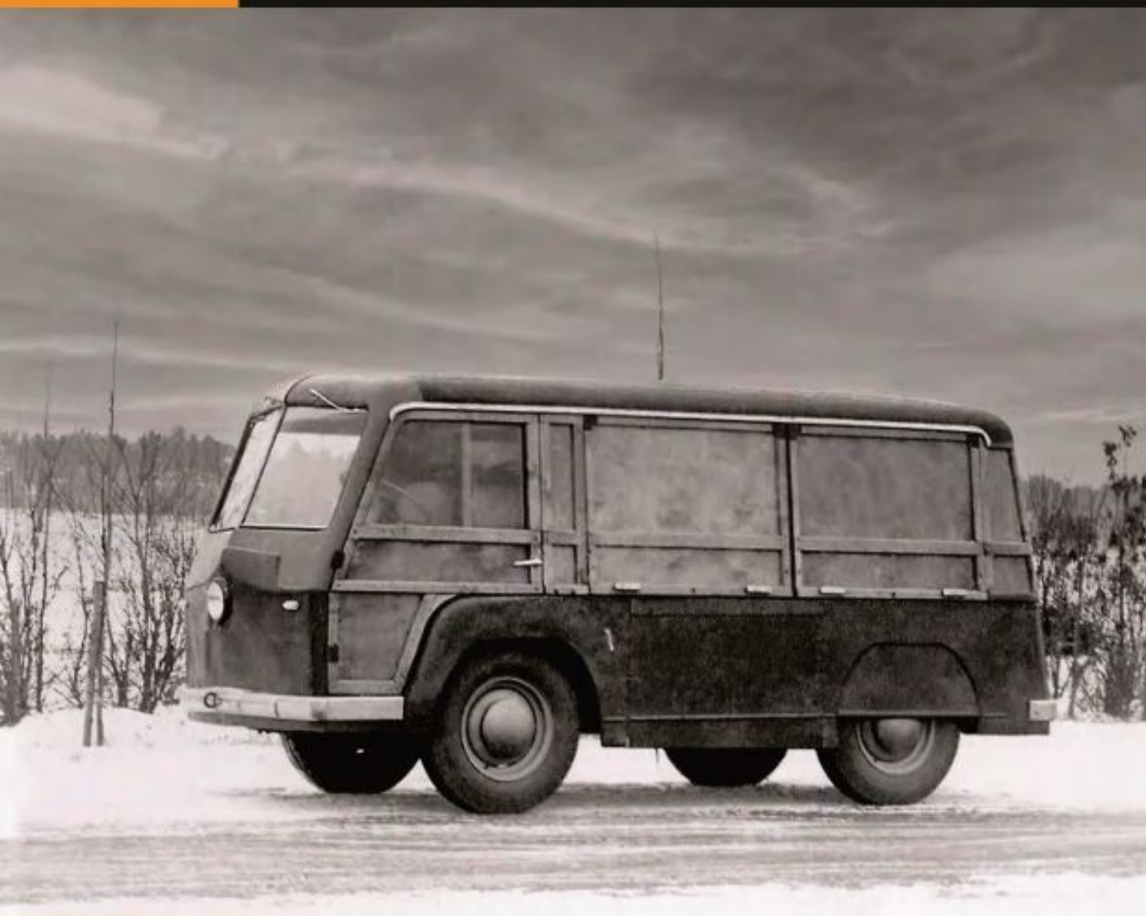
In 1947-1948 NAMI built two electric van prototypes, called the 750 and 751.
