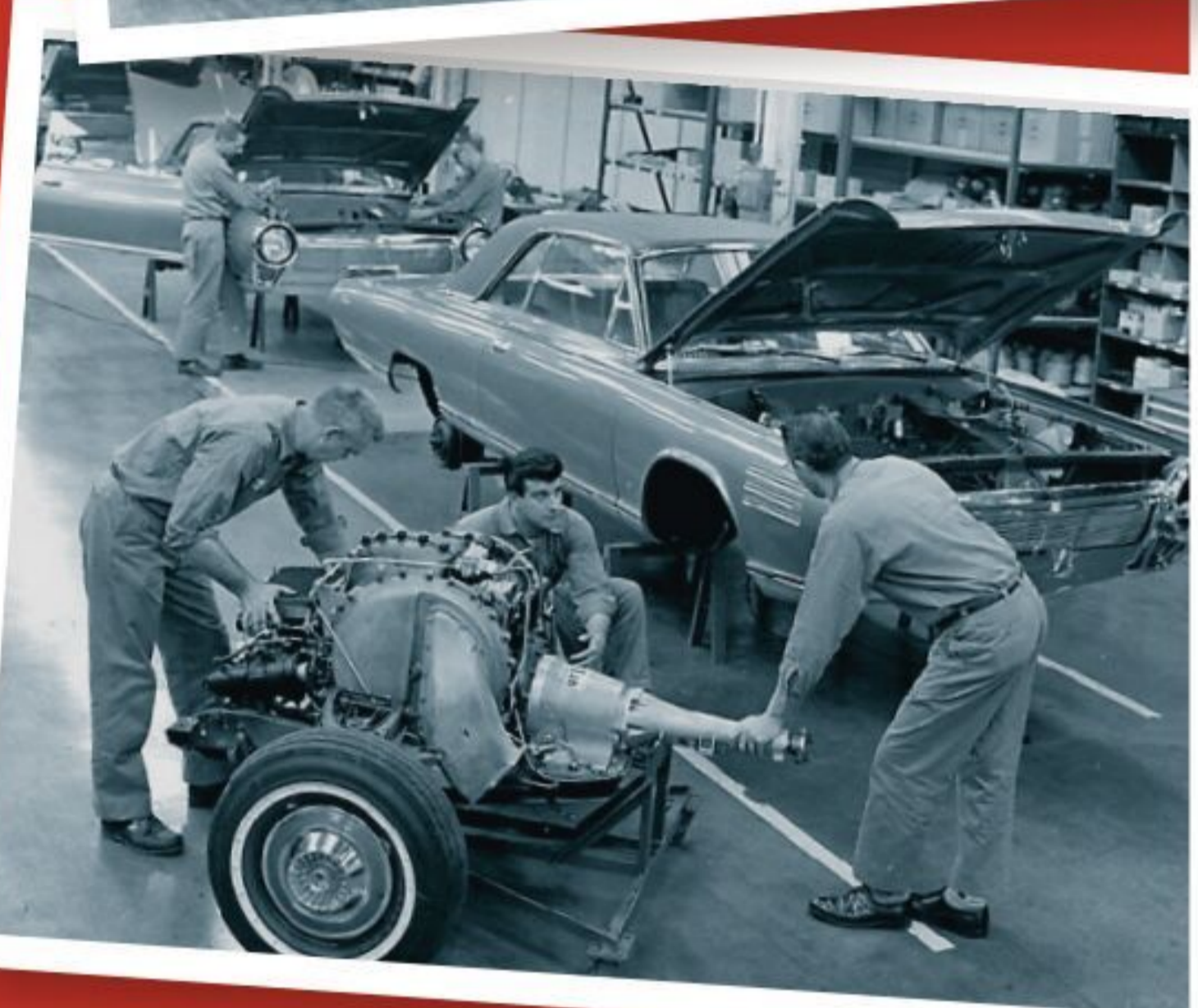
At a dedicated facility in Highland Park, Michigan, the turbine engines and driveline components, such as a modified TorqueFlite three-speed automatic transmission, were installed in the Ghia-built bodies that had been shipped from Turin, Italy (in much the same way as the Cadillac Allanté was assembled, more than 20 years later).
